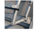
The FlexLink™ forms its own rotating framework at the bottom of the channel.
