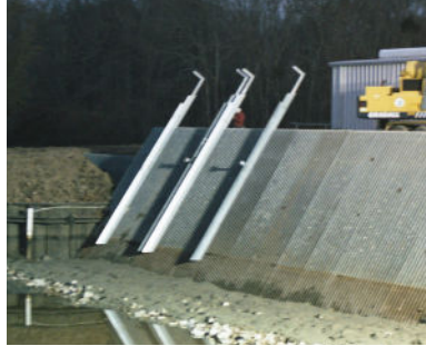
Side fab mounting for Rake Only model
